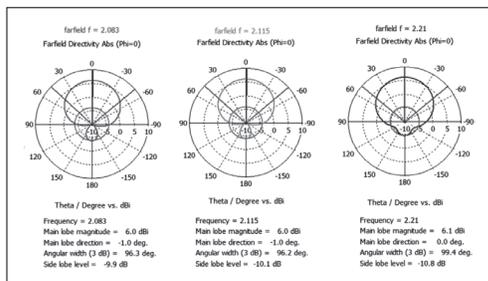
Figure 5: Plot of Radiation Pattern when switch is ON.
