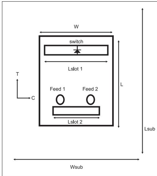
**Figure 1: Proposed reconfigurable antenna with two slots and switch.**
