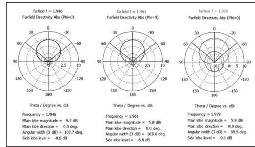
Figure 6: Plot of Radiation Pattern when switch is OFF.
