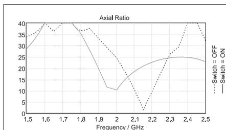
Figure 4: Axial Ratio vs frequency plot for ON/OFF states.
